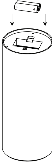
Insert two AA batteries with positive (+) facing positive (+) and negative (-) facing negative (-)
